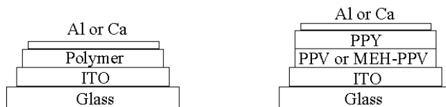
Figure 2. Structure of single and bilayer polymer diodes. The left figure shows the structure of a single layer diode, the polymer layer consisting of PPV, MEH-PPV or PPY, fabricated with aluminium or calcium electrodes. The right panel shows the structure of a bilayer diode.
